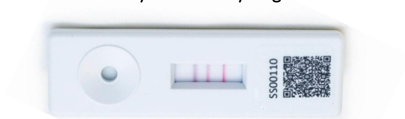
Bild LFA (Lateral Flow Assay), Quelle: www.abingdonhealth.com/contract-services/what-is-a-lateral-flow-immunoassay/
