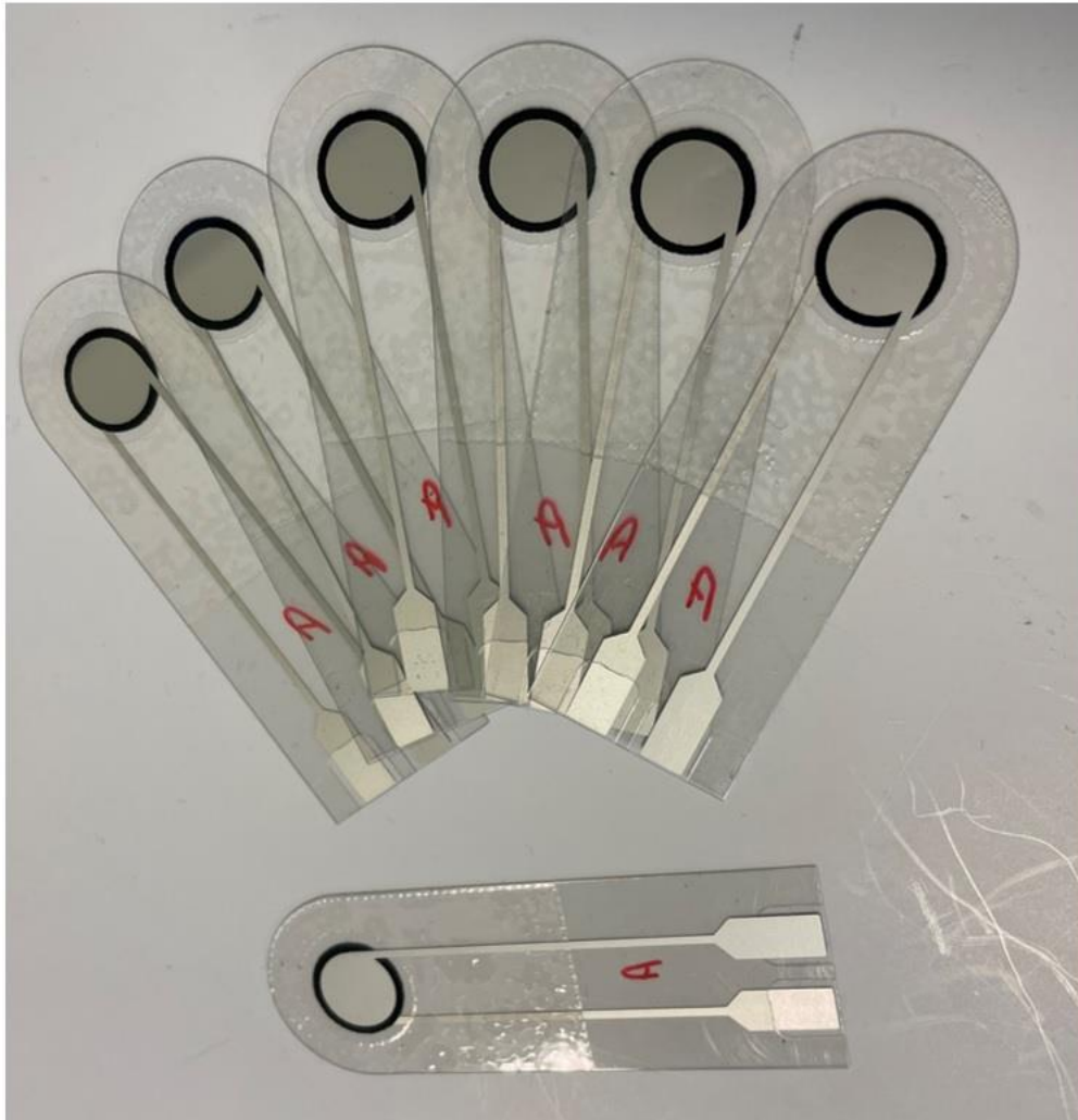
Pressure sensor with contact areas
